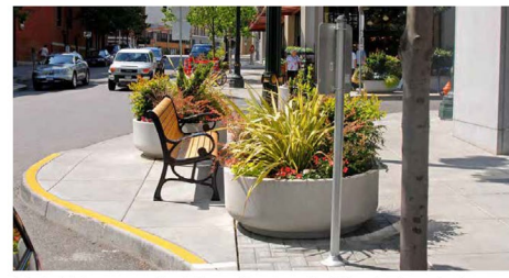
Bulb-outs at street corners can provide pedestrian amenities, such as seating, lighting, and planters on otherwise narrow sidewalks.
