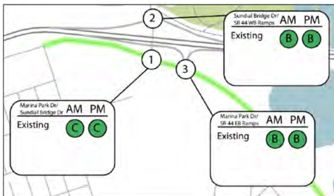
Figure 4.5 Peak Hour Intersection Level of Service (LOS)
